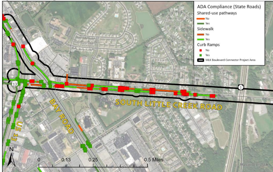
Figure 1: A map showing segments of sidewalk, shared-use pathway, and curb ramps along state-maintained roads, and their designation as Compliant or Non-Compliant by ADA standards.
